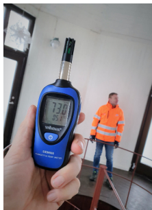
Moisture measurement with hand instrument
