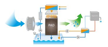
NEXT-S in heating & humidifying mode warming the airflow and increasing the relative humidity level at the same time.
